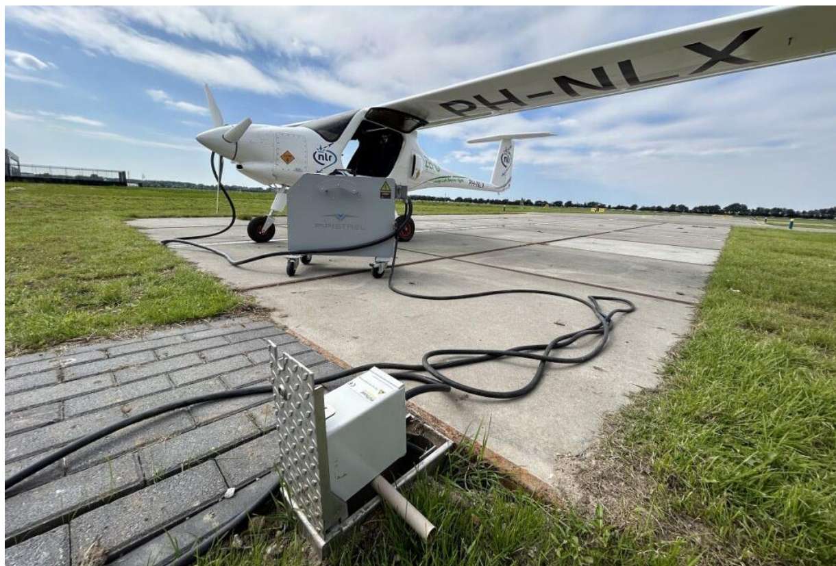
Figure 6 – Charging infrastructure at the demonstration parking stand at Platform Quebec
