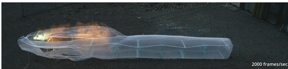
Figure 25 Hydrogen deflagration (WHA international INC., 2023)
