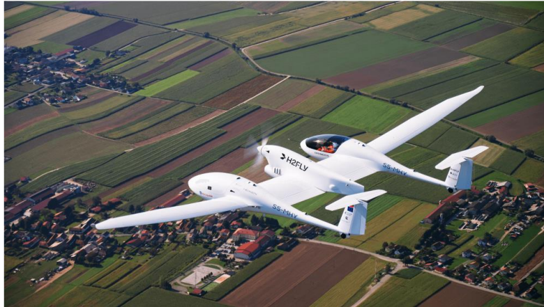
Figure 7 In flight image of the HY4 aircraft powered by a LH2 fuel cell system
