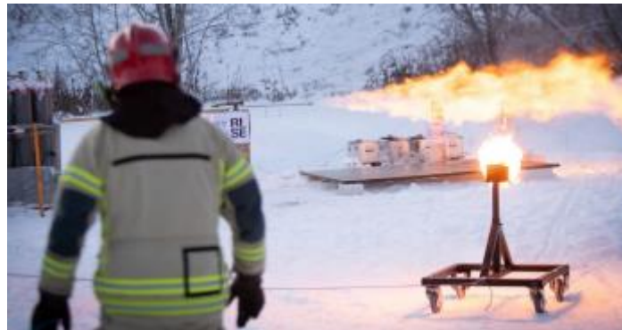
Figure 24 Hydrogen jet fire experiment (Maraner, Stolen, & Li, 2019)
