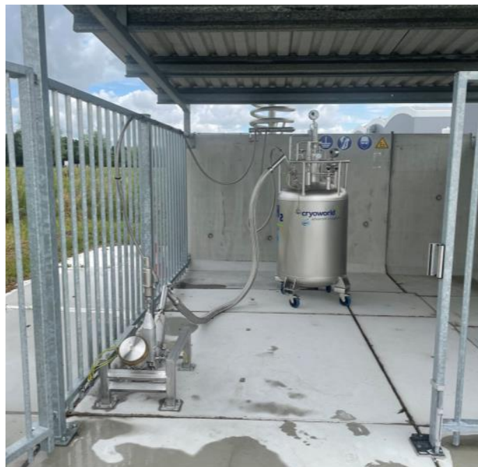
Figure 13 LH2 125L Dewar connected to the filling adapter with the filling hose
