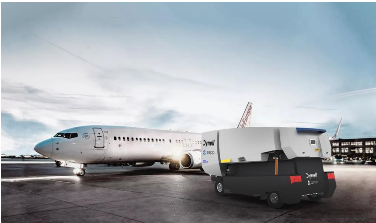
Figure 4: Mobile ground power unit at airside (Dynell, 2023).
