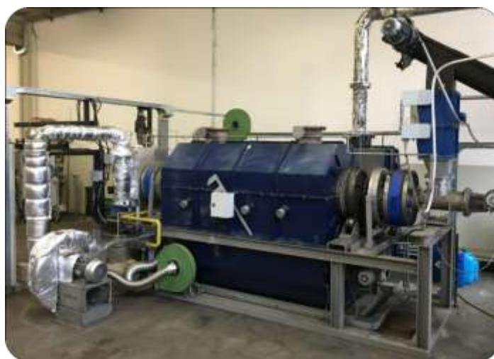
Figure 8: Rotating Kiln at RE-CORD premises used in the TULIPS project
