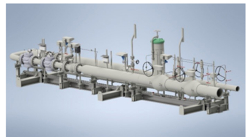
Figure 7 Bilfinger standardised design for hydrogen receiving stations
